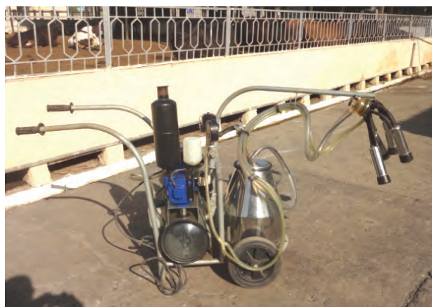
Fig. 3.14(a): A mobile automatic milking machine
